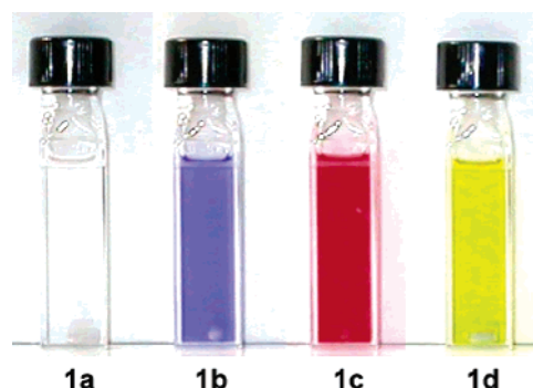
Figure 2. Colors of the open-ring isomer 1a and the isolated closed-ring isomers 1b–d in hexane solution.
